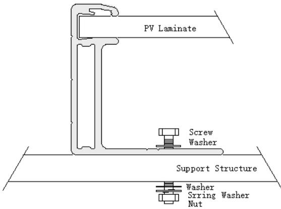
Method B: Use four clamps on the short side. Mounting rails run parallel to the long side frame.
