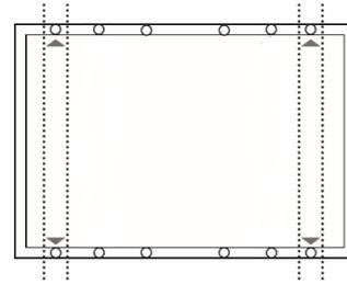
Installed with lateral mounting holes
