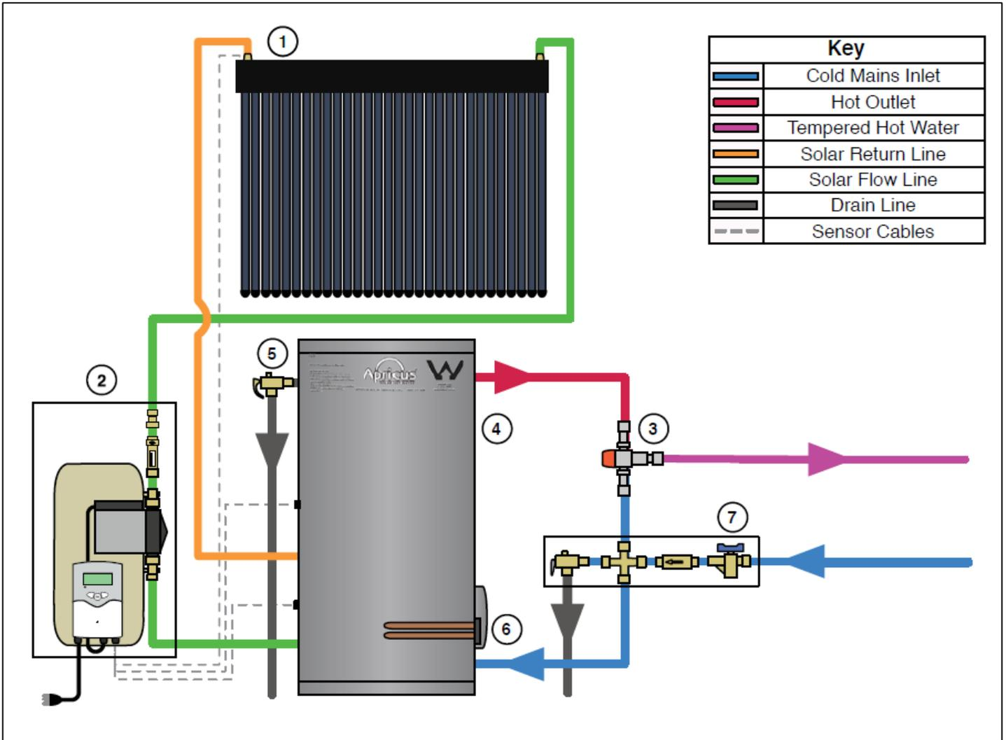
Figure 3 Typical Electric boosted solar hot water system.
