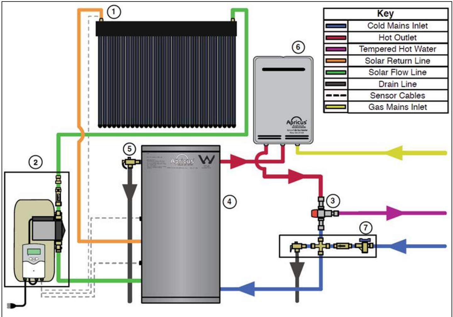
Figure 4 Typical Gas boosted solar hot water system.
